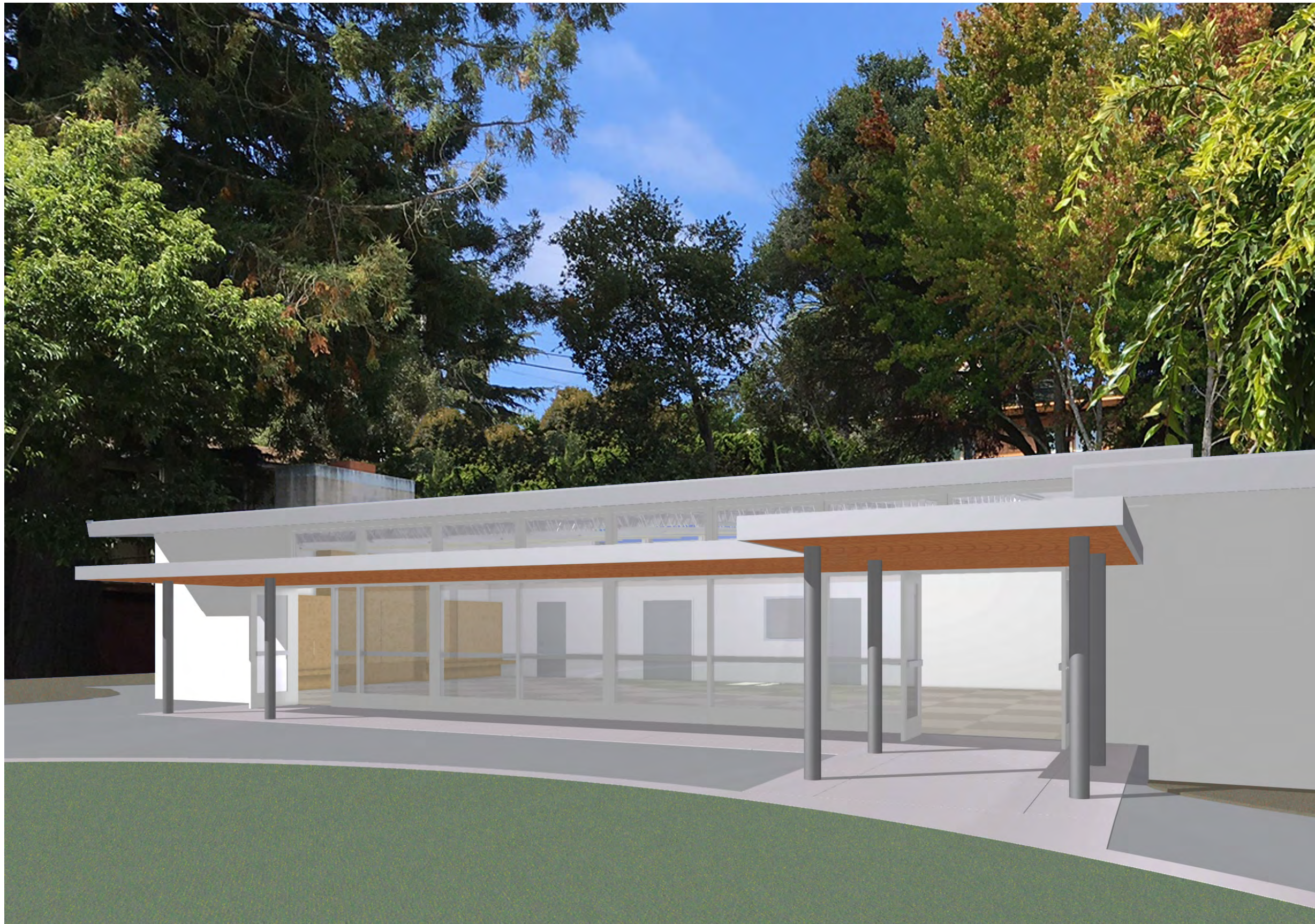
Exterior - New Structural Frame, Canopy and Window Wall with Fixed Windows
