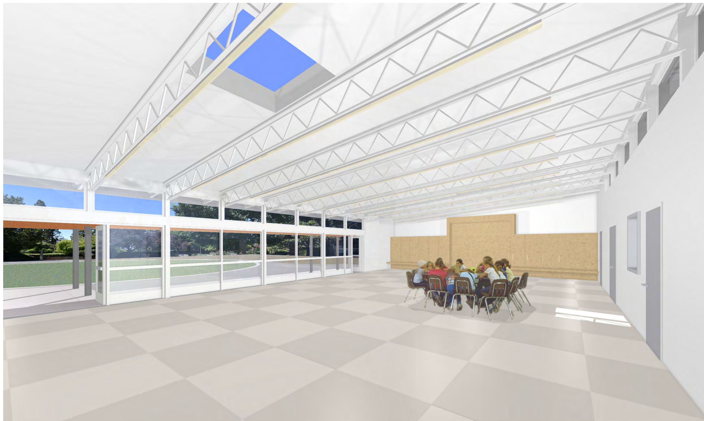
Interior - New Structural Frame, Canopy and Window Wall with Fixed Windows
